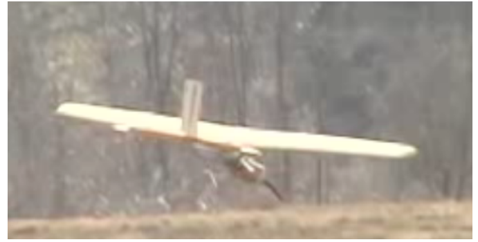
Figure 18: Flight test with warping wing.
