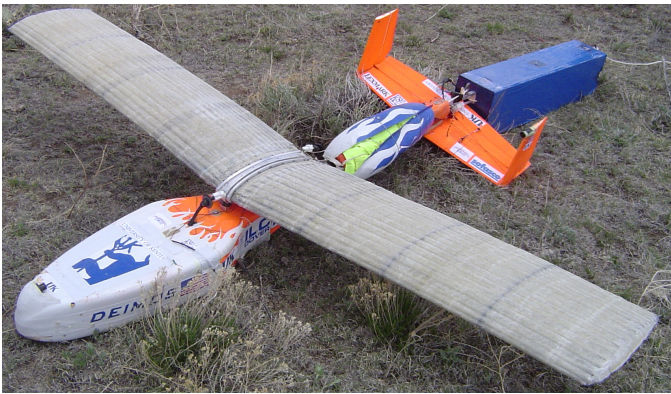
Figure 6: Recovery of second-generation inflatable/rigidizable high-altitude test article.
