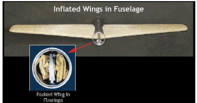
Figure 5: ILC Dovers multi-spar Inflated wing and packed configuration.
