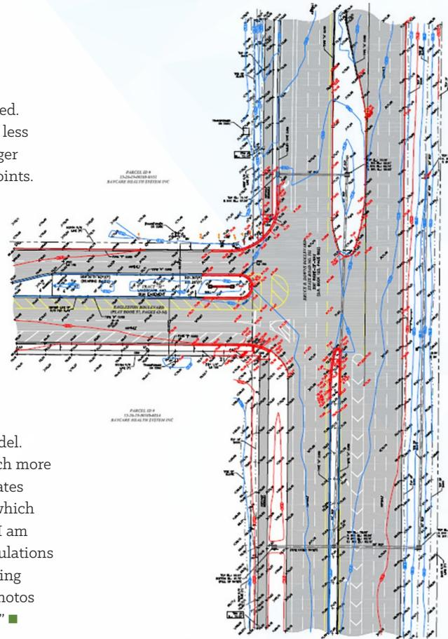
This resulting map was created using Photomodeler. An entire second set of data was acquired using conventional methods as a comparison. On average, a difference of less than 0.1' was observed between the elevations of asphalt and concrete established by Photomodeler and the conventional data.
