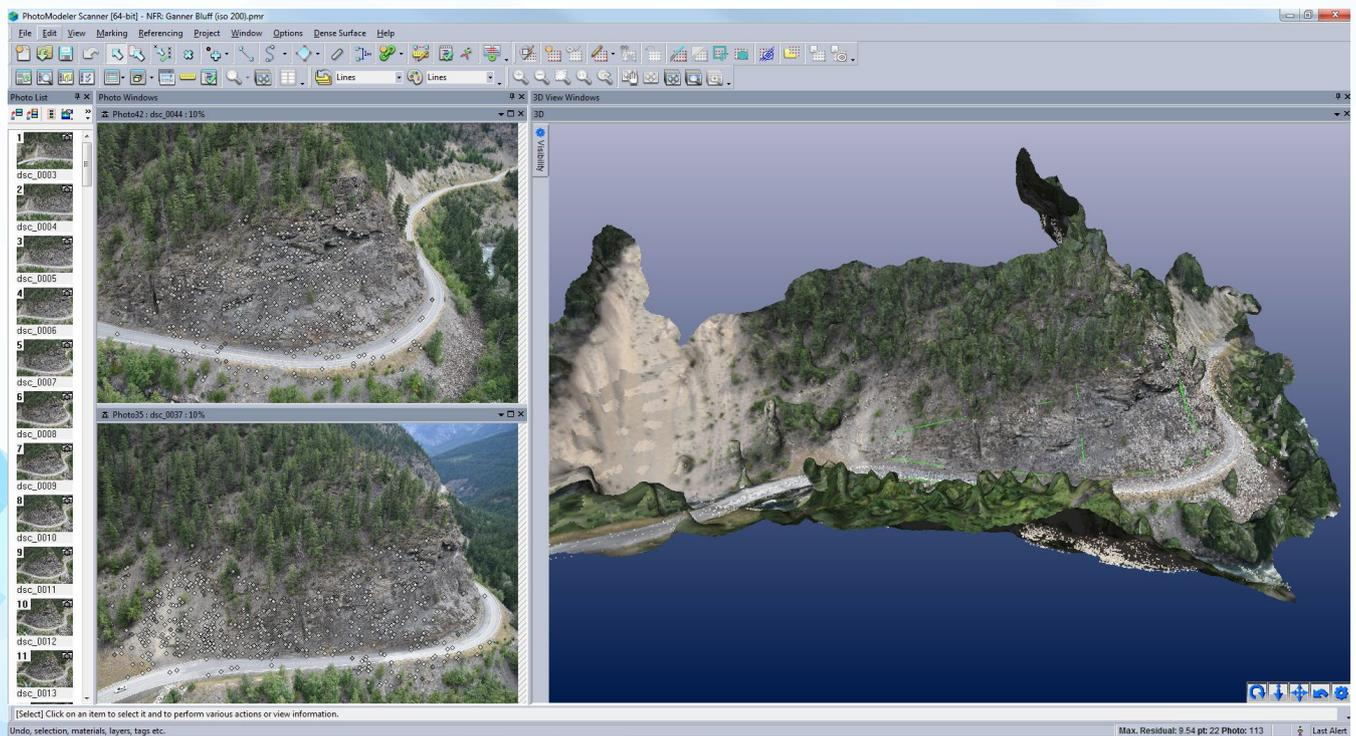
Rendered 3D surface model (right) of the bluff in previous image. The individual photos taken at the site are shown in the two images on the left. PhotoModeler surface drawing tools were used to outline the area of proposed slope mesh (green lines on surface model). The surface model with 3D lines outlining proposed slope mesh areas are imported into AutoCAD Civil 3D to calculate mesh surface areas and produce final drawings.
