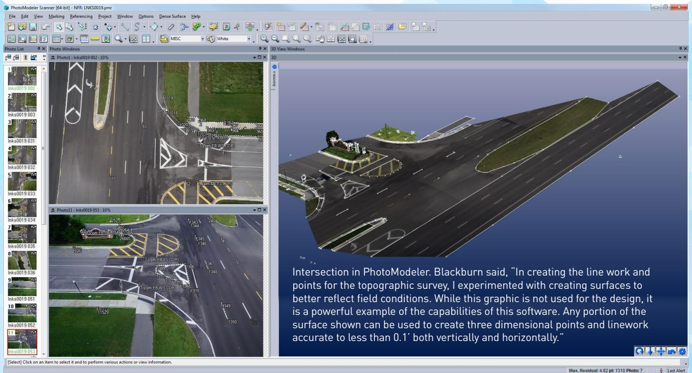
Intersection in PhotoModeler. Blackburn said, "In creating the line work and points for the topographic survey, I experimented with creating surfaces to better reflect field conditions. While this graphic is not used for the design, it is a powerful example of the capabilities of this software. Any portion of the surface shown can be used to create three dimensional points and linework accurate to less than 0.1' both vertically and horizontally."
