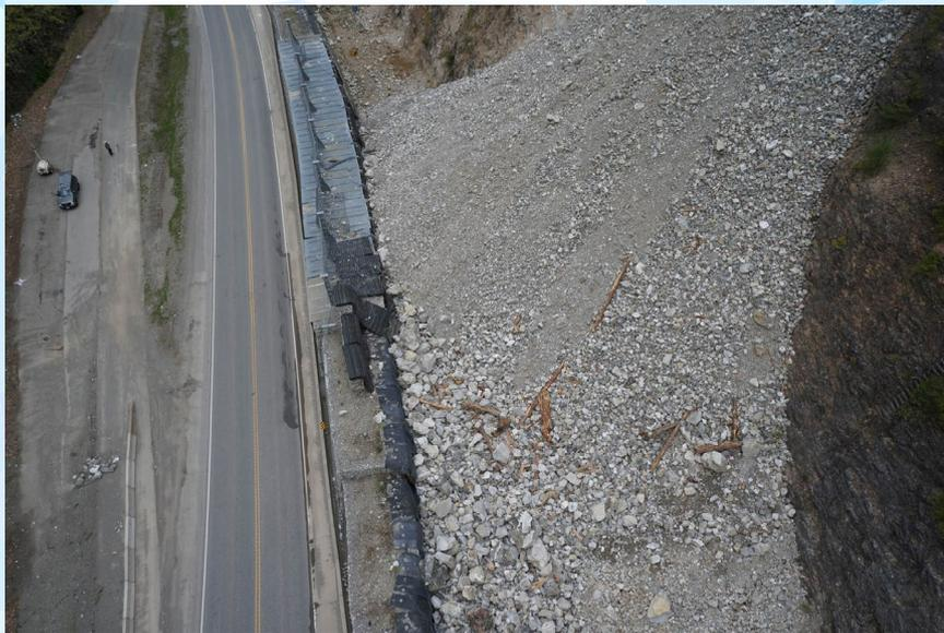
Aerial view of a debris slide catchment area. This photo shows the catchment area before the contractor has removed the debris and is one of many that will be imported into PhotoModeler to calculate the total debris volume of the slide.
