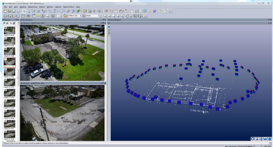
Bank site in PhotoModeler. On the right is the set of georeferenced 3D point locations which will be exported to AutoCAD software. Two of the 40+ images taken of the survey site can be seen on the left.
