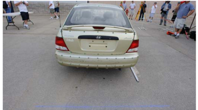
Figure 4. Accent rear damage, measurement points and station line
