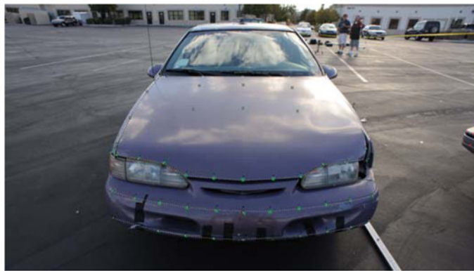
Figure 2. Thunderbird front damage and measurement points
