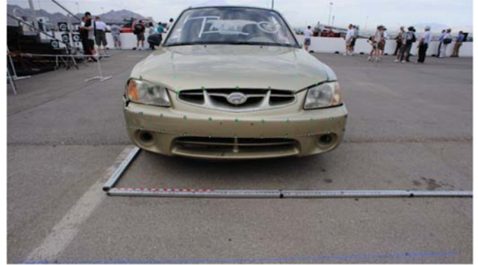
Figure 3. Accent front damage, measurement points and station line
