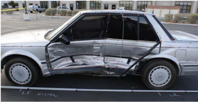
Figure 1. Maxima driver's side damage and measurement points
