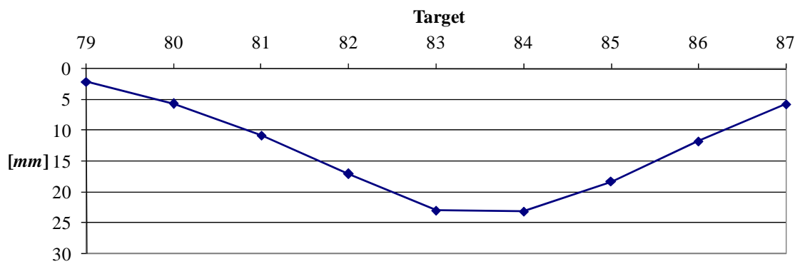
Fig. 8 Vertical displacements for SE loading situation.
